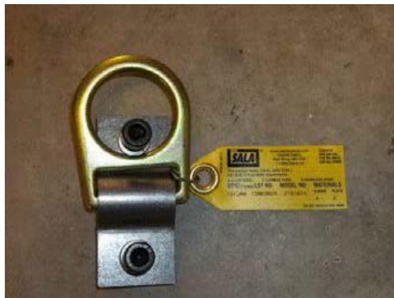
Figure 6 Two-bolt D-ring Anchor Plate attached with ½"-13 TPI UNC 1-1/2" long grade 8 socket head cap screws and lock washers (torque to 40 foot-lbs.)
